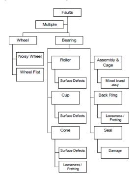
Figure 5. Bearing and wheel fault hierarchy (Southern, Rennison, and Kopke, 2004)
