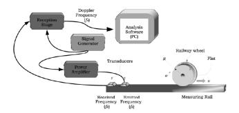
Figure 12. Wheel flat detector prototype (Brizuela et al., 2010)
