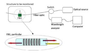
Figure 10. Schematic of the FBG sensor (Roveri et al., 2015)
