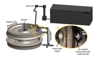
Figure 7. The laser-ultrasonic experimental set-up (Cavuto et al., 2016)
