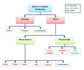
Figure 14. Overview of available CM technologies for railway bearing and wheel health monitoring
