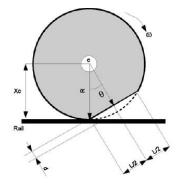
Figure 11. Simplified wheel flat measurement model (Brizuela et al., 2010)
