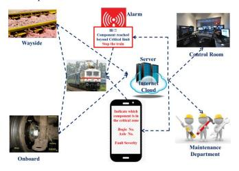
Figure 6. CBM architecture for railway
