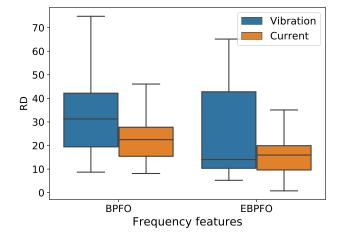
Figure 4. Comparison between features in frequency domain, BOF, HS: 2880 rpm.
