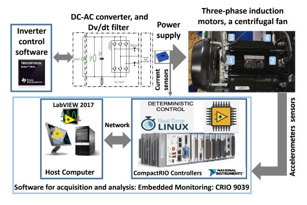
Figure 2. Experimental system configuration.
